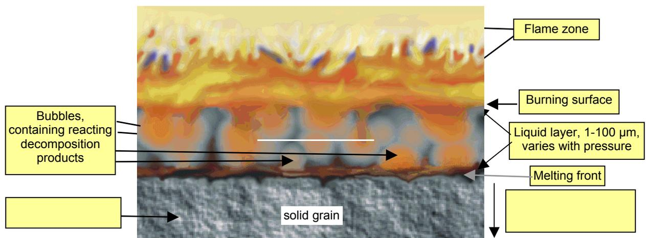
**Picture 70: Burning Surface of Propellant Granule**
