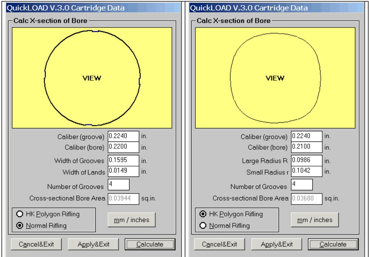
**Picture 28: Cartridge data – Selecting *Calc* X-section of bore:**
