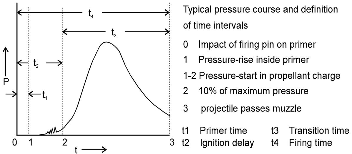
**Picture 67: Typical Pressure Curve Inside the Combustion Chamber**
