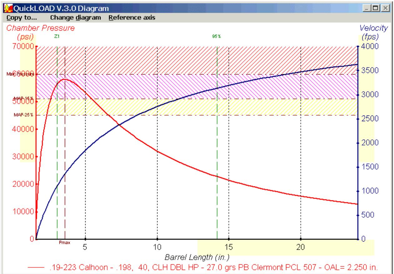
**Picture 62: Diagram Velocity and Pressure vs. Barrel length**
