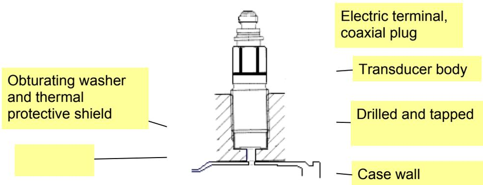
**Picture 68: Transducer mounted into Chamber Wall**
