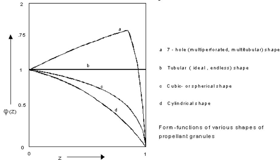
**Picture 72: Shapes of Powder's Geometric Form Functions**
