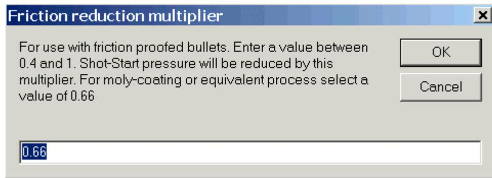
**Picture 51: Friction reduction multiplier entry**
