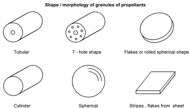
**Picture 71: Examples of Smokeless Propellants, Granule Form.**
