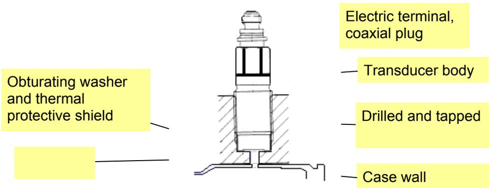
**Picture 68: Transducer mounted into Chamber Wall**
