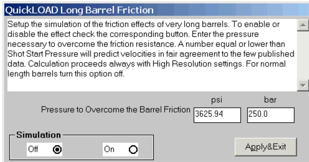
**Picture 16: Set Long Barrel Friction**
