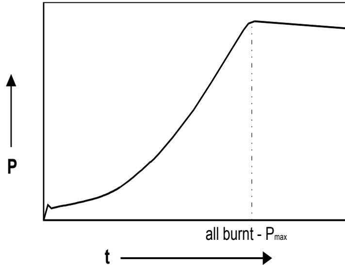
Picture 73: Pressure curve from closed bomb
